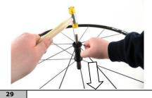
Take care to ensure that the cup stripper and punch are not propelled out of the hub when finally free of the hub shell.
