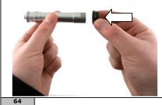
Insert the adjustment cone on the axle.
