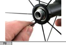
Manipulate it into position by using a small screwdriver. Push the adjustment cone in by pressing on various points of the circumference.
