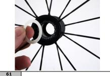
The black part of the grease seal should face the inside of the hub's body.
