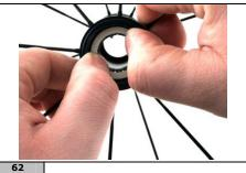
Insert the grease seal inside the corresponding notch in the cup of the hub.
