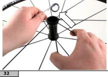
Remove the grease shields on both sides.
