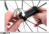
Install and tighten the adjustment ring nut clockwise and hold the axle while holding the axle stationary with your right hand.
