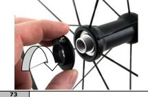
Inspect the adjustment ring nut. If it is damaged, replace it.
