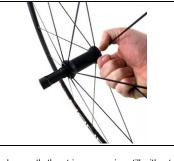
Once inserted correctly the stripper remains still without operator assistance. Rotate the hub in the opposite direction.
