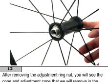
After removing the adjustment ring nut, you will see the cone and adjustment cone that we will remove in the next stage.
