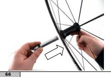
Insert the axle inside the right side of the hub body.
