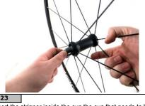
Insert the stripper inside the cup the cup that needs to be removed.
