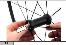
Push the axle into the hub body until it reaches the other side.
