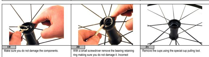
handling may cause the bearings to detach from the ring.
