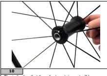
The indication that the adjustment ring nut will be loosened will be when the slot in the nut has a visible gap. Do not remove the screw from the adjustment ring nut.
