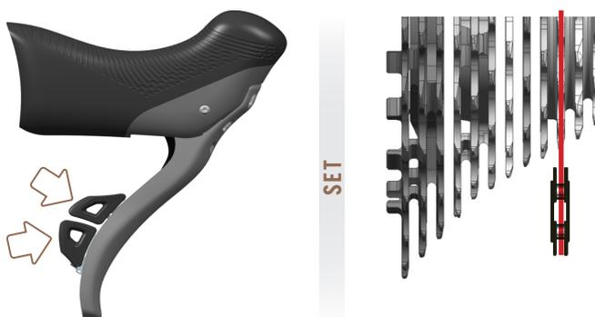
4) Press the rear derailleur MODE button to confirm the position.
