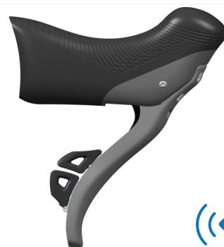
The LED remains flashing in high frequency until the control is coupled to the rear derailleur: if after **90 s** it continues to flash, and therefore it is not coupled, the LED turns off.
