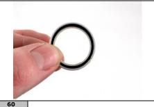
The hub shield must be undamaged. Replace if damaged.
