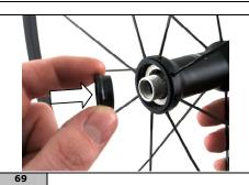
Insert the second cone onto the axle following the direction it should be inserted in. The larger diameter should face the outside of the hub's body.
