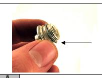
While removing the end cap, make sure you do not lose the spacer.
