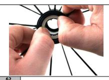
Insert the grease seal inside the corresponding notch in the cup of the hub.
