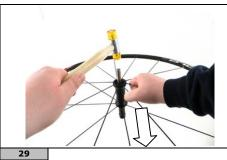
Take care to ensure that the cup stripper and punch are not propelled out of the hub when finally free of the hub shell.
