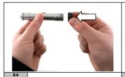
Insert the adjustment cone on the axle.
