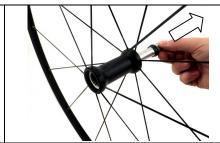
Remove the cone from the axle.
