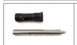
The cup pulling tool consists of two items. A specific stripper for road cups and a punch.
