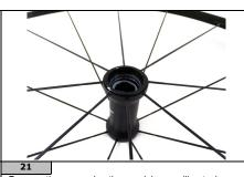
Remove the cups using the special cup pulling tool.
