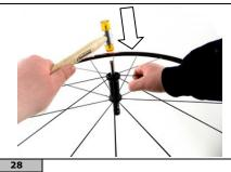
Continue to deliver blows to the punch until the cup is removed from the hub shell.
