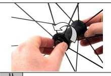
Holding the axle stationary, rotate the adjustment ring nut counter-clockwise to remove the adjustment ring nut.
