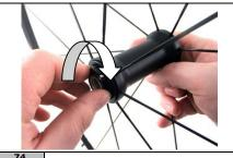
Install and tighten the adjustment ring nut clockwise and hold the axle while holding the axle stationary with your right hand.
