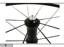
Using 2, 5mm hex wrenches to loosen the axles end-cap/flange.
