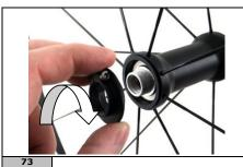
Inspect the adjustment ring nut. If it is damaged, replace
