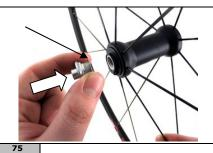
Inspect the axle end cap. If it is damaged, replace it. Insure that the small spacer is in place and install the end cap into the axle end.
