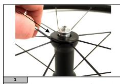
With a flat-bladed screwdriver remove the first protective cover. Make sure you do not damage the cover's locking teeth which would affect reassembling at a later stage.
