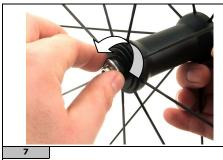
Loosen end cap (adjustment ring nut side).
