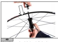
Insert the second cup/adaptor onto the bearing press tool.
