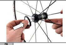
Inspect the dust covers. If they are damaged, replace them. Insert the cover with the larger internal diameter on the body of the hub on the adjustment ring nut side.
