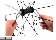
Insert the two hex wrenches inside the hex-drive of the Of the axle and end cap then firmly unscrew. The right side (on the opposite side of the adjustment ring nut) remains fixed, the left side end cap rotates counterclockwise to loosen the end cap.
