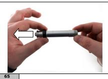
Ensure that the cone seats properly onto the corresponding cone shape on the axle.
