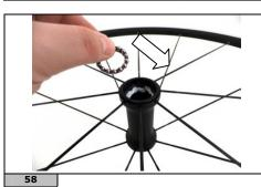
Insert the bearing retaining ring inside the cups body of the hub.
