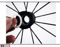
The black part of the grease seal should face the inside of the hub's body.
