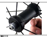
Make sure the cover engages correctly into place.
