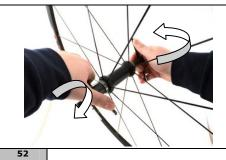
Firmly close the two handles of the tool until the cups are fully inserted.
