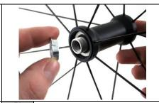
Insert the adjustment cone onto the axle mating into the cone from 69-70. The direction it should be inserted in. The larger diameter should face the outside of the hub's body.
