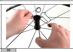
Remove the grease shields on both sides.
