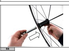
Insert the axle inside the right side of the hub body.
