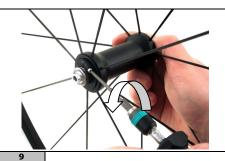
Use a screwdriver with a 2.5mm hexagon insert to loosen the screw of the adjustment ring nut.
