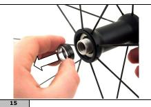
Remove the cone and the adjustment cone.
