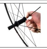
Once inserted correctly the stripper remains still without operator assistance. Rotate the hub in the opposite direction.
