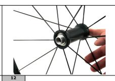
After removing the adjustment ring nut, you will see the cone and adjustment cone that we will remove in the next stage.
