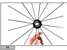
When removing the cups the grease shields may move away from their housings.
