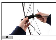
Remove the tool from the hub shell.
