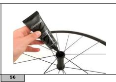
Grease the surface of the cup ball race using specific grease for bearings.
