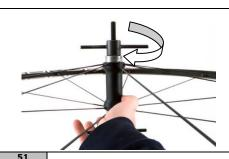
Screw on the threaded handle to the bearing press tool.
