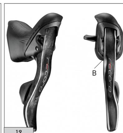
Insert the front derailleur cable (length 1,600 mm -  $\varnothing$  1.2 mm) into the bottom of the control (B - Fig. 19)
