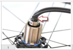
Insert the tool (  $\mbox{\bf UT-WHDB001}$  or  $\mbox{\bf UT-WHDB002})$  on the right of the axle.
