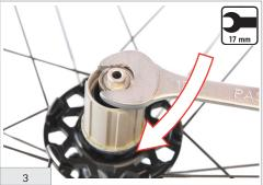
Apply a 17 mm spanner on the right side of the axle and loosen the nut (Attention! The nut is left-threaded).
