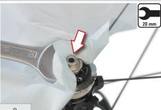
Place a 20 mm spanner on the adjustment ring nut, protecting it with workshop paper in order not to scrape it.
