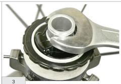
Lock the axle in place with a 14 mm spanner.
