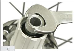
Unscrew the nut on the FW body. Attention: left hand thread!
