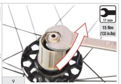
Apply a 17 mm spanner on the right side of the axle and tighten the nut to a torque of 15 Nm (133 in.lbs) (Attention! The nut is left-threaded).
