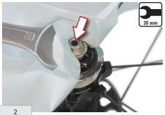
Place a fixed 20 mm spanner on the adjustment ring nut, protecting it with workshop paper in order not to scrape it.
