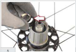
Remove the nut and the spacer.
