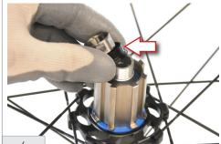
Insert the spacer and tighten the nut (Attention! The nut is left-threaded).
