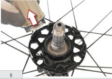
Remove the FW body from the hub axle.
