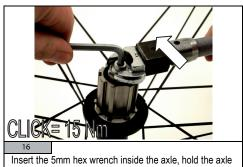
stationary and torque the lock nut with the a 17mm crows foot and a torque wrench.
