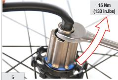
Insert the tool (**UT-WHDB001** or **UT-WHDB002**) on the right of the axle. Using an 18 mm spanner, tighten to a torque of **15 Nm (133 in.lbs)**.
