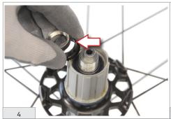
Remove the nut and the spacer.
