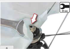
Place a 20 mm spanner on the adjustment ring nut, protecting it with workshop paper in order not to scrape it.
