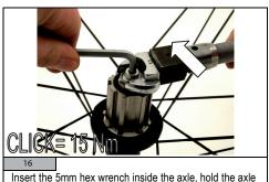
Insert the 5mm hex wrench inside the axle, hold the axle stationary and torque the lock nut with the a 17mm crows foot and a torque wrench.
