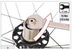
Apply a 17 mm spanner on the right side of the axle and tighten the nut to a torque of **15 Nm (133 in.lbs)** (Attention! The nut is left-threaded).
