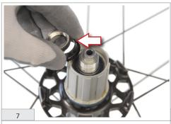
Insert the spacer and tighten the nut (Attention! The nut is left-threaded).
