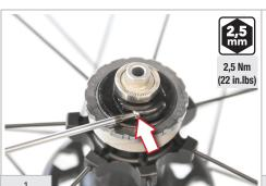
Using a 2.5 mm Allen wrench, ensure that the clearance recovery ring nut is tightened (screw tightened to **2.5 Nm - 22 in.lbs**) so that the ring nut does not turn.
