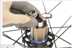
Insert the spacer and tighten the nut (Attention! The nut is left-threaded).
