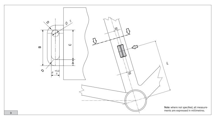
In order to have compatibility with all the chainrings indicated in table 1, the following measurements must be observed: C: minimum value 22 mm (C > 22 mm) - B: maximum value 27 mm (B < 27 mm) - A: maximum value 5 mm.
