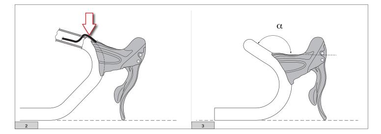
WARNING: The cable routing illustrated in Figure 2 seriously compromises the drivetrain's gear shift and derailing performance. DO NOT USE HANDLEBAR BENDS WITH THIS KIND OF ROUTING.
