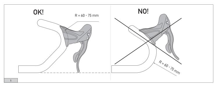
• Do not lodge the upper part of the command in the rectilinear section of the handlebar (Fig. 1).
