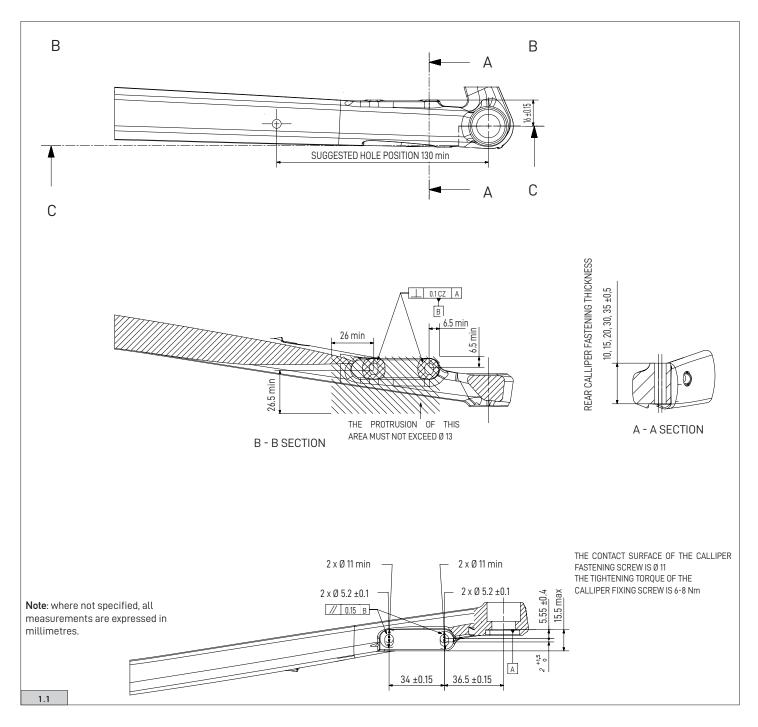
• Using the frame cutter tool make sure the calliper contact surface on the fork and the left-hand chain stay are perpendicular to the discs, grinding the frame if necessary in order to achieve this (Fig. 2).
