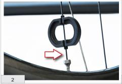
Position the spoke anti-rotation tool in the corresponding spoke.
