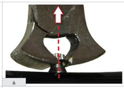
Insert the nipple through the valve hole.
