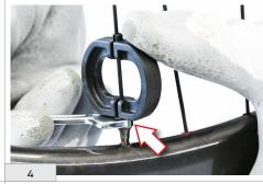
Maintaining pressure on the spoke anti-rotation tool and keeping it in place, turn the nipple torx insert with an 8 mm fixed wrench.
