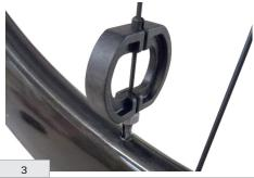
Lower the spoke anti-rotation tool and insert the guide cylinder into the nipple torx insert.
